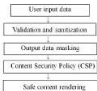
Fig. 1. Concept of protection against XSS attacks
