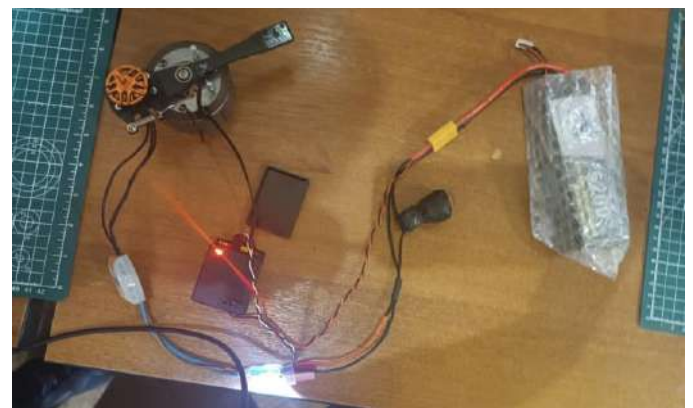
Fig. 1. Working model of the brushless DC motors quality assessment stand
